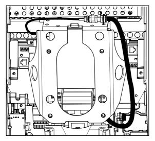
Figure 12: Connecting the television cable
